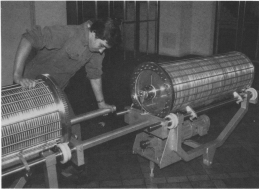
Fig. 17. Assembling two cylinders, pilot-scale extractor. Volume, 250 l; feed \leq 25 l; explosion-proof motor underneath, other accessories located in a separate room; movable.
